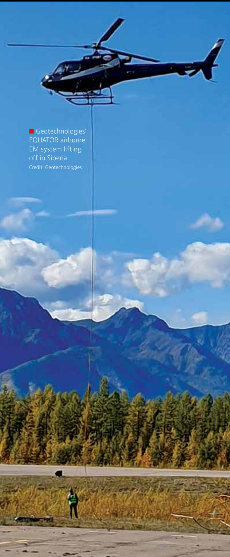
■ Geotechnologies' EQUATOR airborne EM system lifting off in Siberia.
