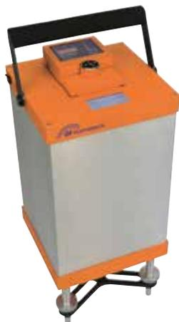
■ GF Instruments' Galileo land gravity meter.
