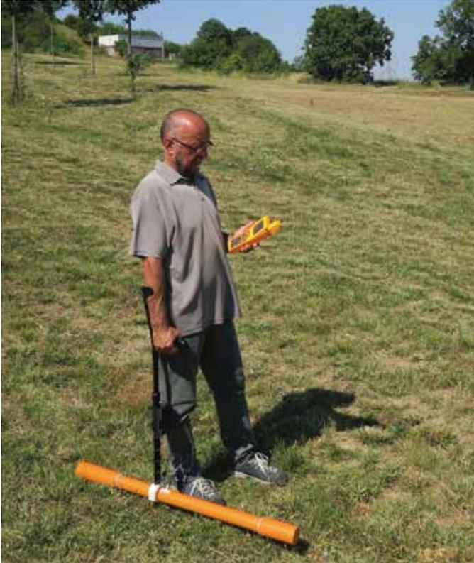
■ GF Instruments' CMD-1 conductivity meter in the field.
