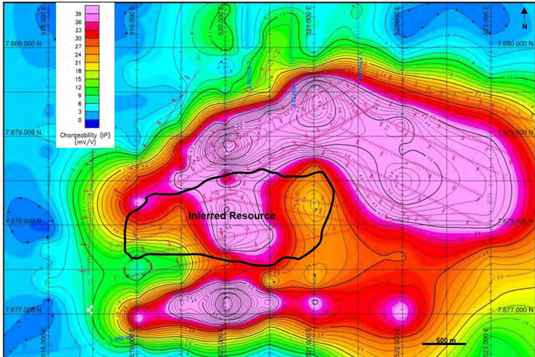
Figure 9. QB chargeability anomaly at 4100 meter elevation.
