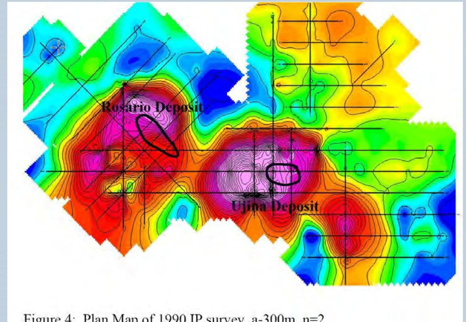
Figure 4: Plan Map of 1990 IP survey, a-300m, n=2
