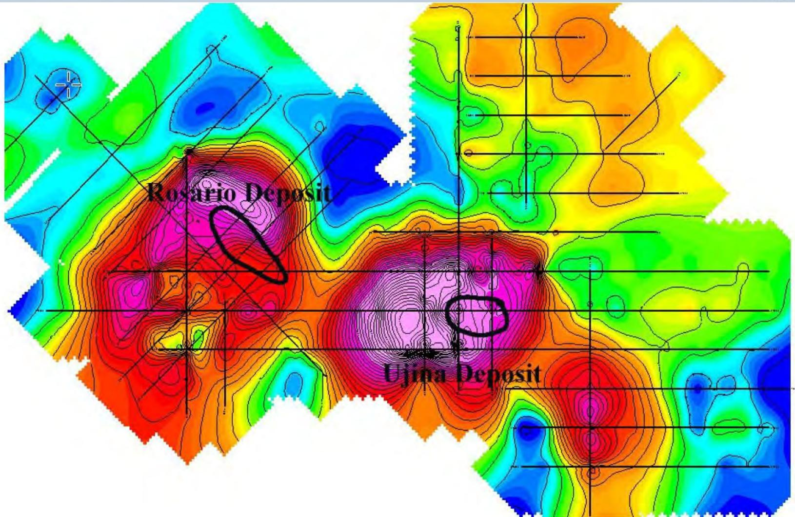
Figure 4: Plan Map of 1990 IP survey, a-300m, n=2
